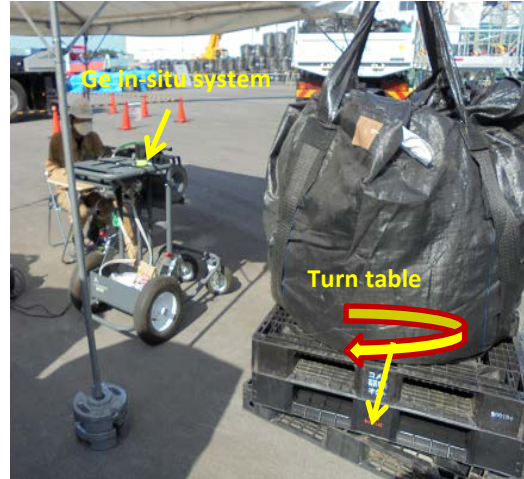
Fig.5 The Ge in-situ measurement station; the average of 4 measurements at 90 degrees was used.
