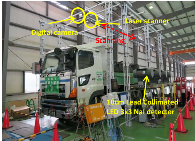
Fig.4 The MTSCAN installation
